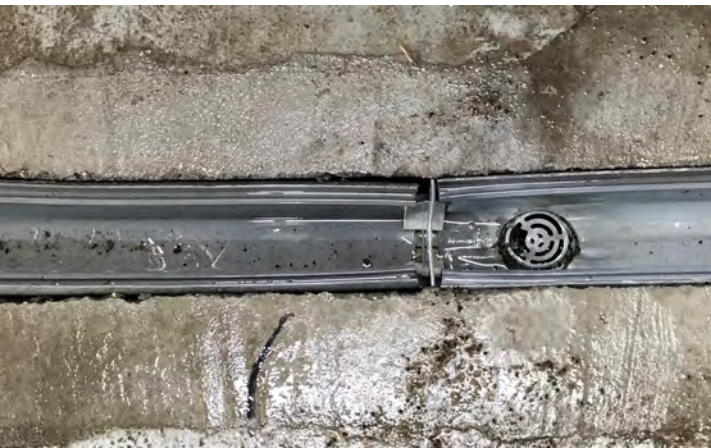
Plastic trench drain after one year of exposure to hot water in a brewery.
